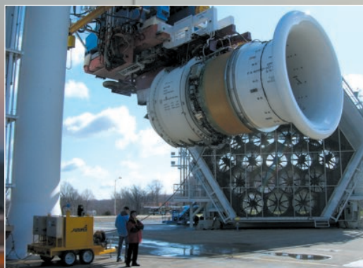
Juniper's new Water Wash Cart being used for the first time on a GP7200 engine at the GE Peebles Test Operation in rural Southern Ohio
