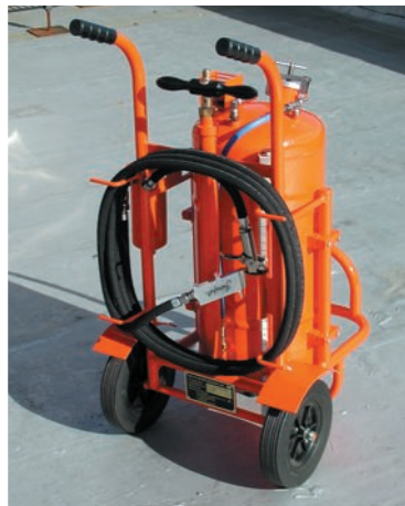
Engine Oil Top Up and Replenishment Rig
