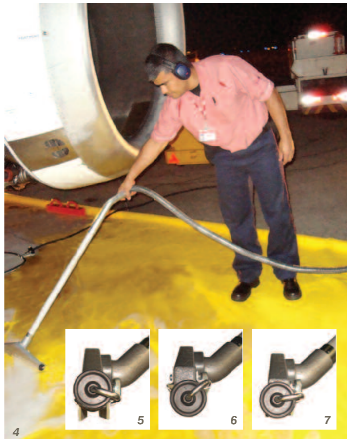
1 Juniper's 2x25 gallon wash rig (JMP/CFM56/D/4777/C200) in the livery of TAM Linhas Aereas being used with the new Kyoto Containment Mat to wash the V2500 engine fitted to an Airbus A320 at the Jardim Aeroporto, San Paulo, Brazil in February 2010
