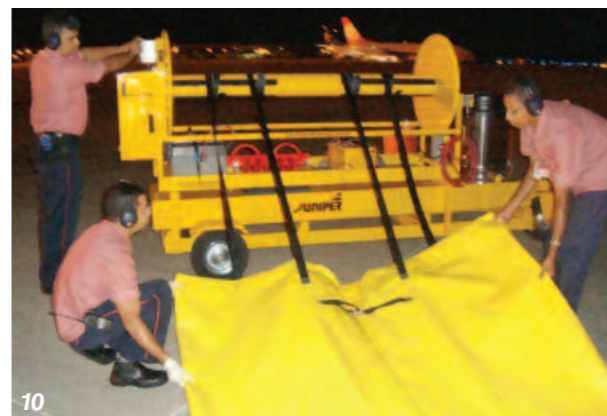
9 The Kyoto Containment Mat in position during a recent engine wash for Aegean Airlines on a V2500 engine fitted to one of their Airbus A320 aircraft. The flexible vacuum hose is connected and ready for use.
