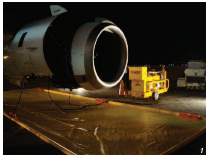
1 Juniper's 2x25 gallon wash rig (JMP/CFM56/D/4777/C200) in the livery of TAM Linhas Aereas being used with the new Kyoto Containment Mat to wash the V2500 engine fitted to an Airbus A320 at the Jardim Aeroporto, San Paulo, Brazil in February 2010
