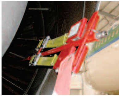
Left and Below Left: Juniper CF6-80E1 long probes in a typical installation on an Airbus A330
